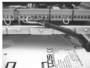
Figure 2 - Correct Screening Method (Tails Kept Short)
