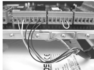
Figure 1 - Incorrect Screening Method (Tails Left Long)
