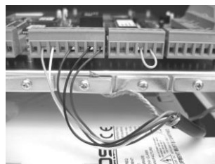
Figure 1 - Incorrect Screening Method (Tails Left Long)
