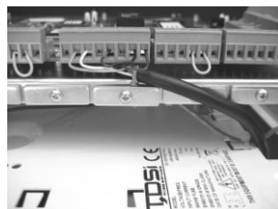
Figure 2 - Correct Screening Method (Tails Kept Short)
